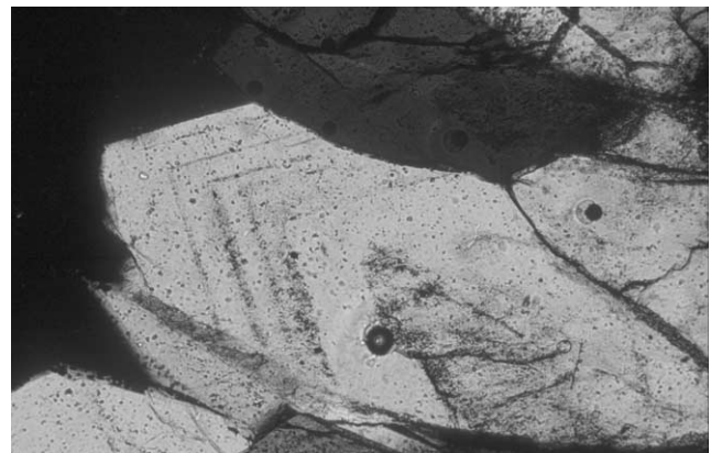
Fig. 3. Photomicrograph of a quartz crystal from the fracture filling. Growth zonation is marked by planes of fluid inclusions parallel to the rhombohedral faces of the quartz crystal against an open cavity. Long side of photomicrograph = 1.02 mm. Crossed polarizers.
